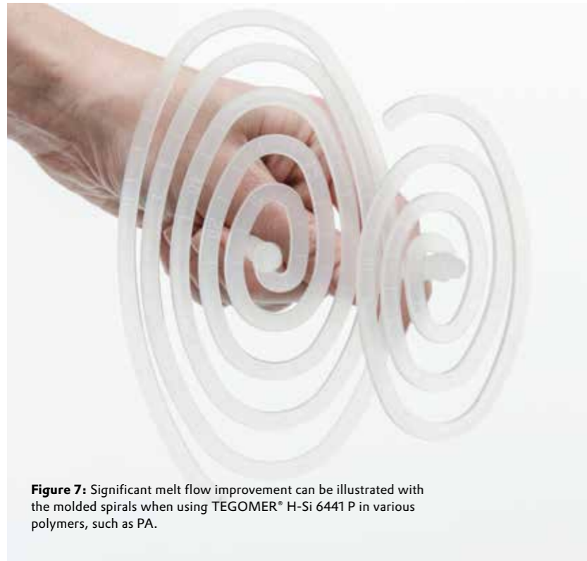
Figure 6: Improvement of melt flow path by TEGOMER® H-Si 6441 P
