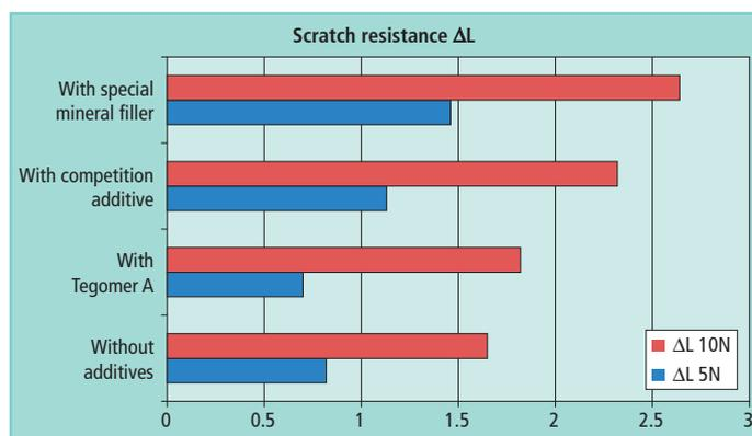
Fig. 9: Results of the abrasion resistance test (ASTM D5963)
