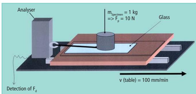
**Fig. 2:** Measuring the dynamic coefficient of friction
