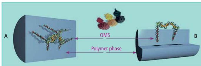
Fig. 5: Functionalization of a polymer matrix with OMS (A = bulk modification, B = surface modification)
