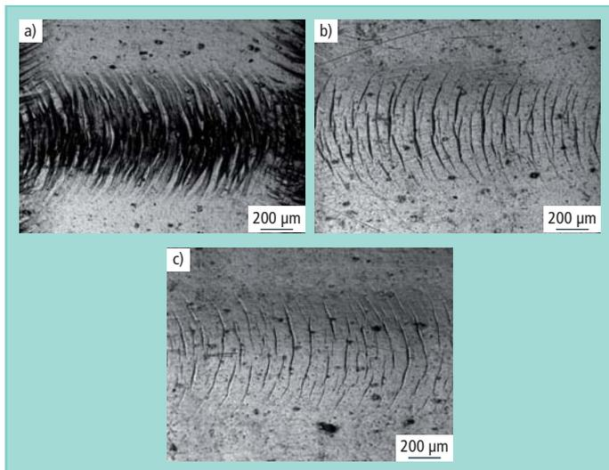
Fig. 6: Effect of siloxanes in a SEBS compound
