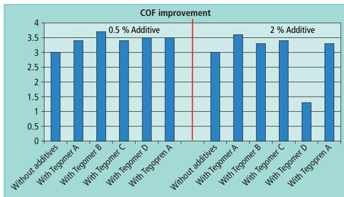
Fig. 13: Results of the abrasion resistance test (ASTM D5963)
