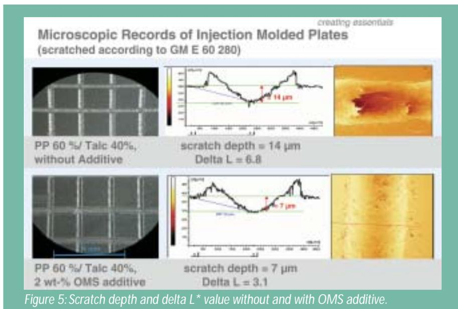
Figure 5: Scratch depth and delta L\* value without and with OMS additive.
