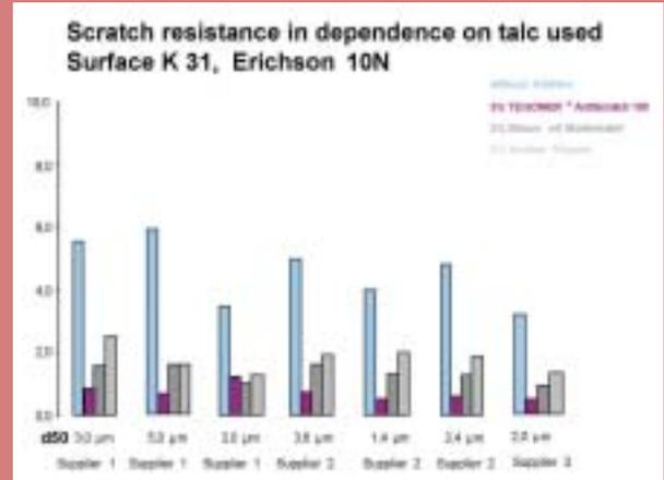
Figure 7: Different talc grades in a 18% talc filled copolymer, surface K 31.
