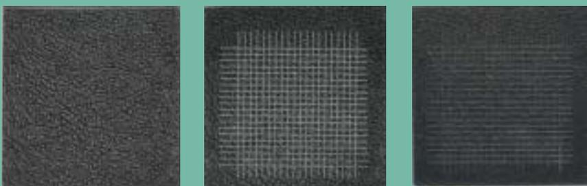
Figure 4: Unscratched surface (left), scratched without additive (centre) and scratched with additive (right).
