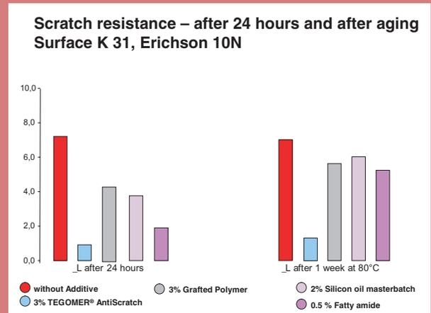
Figure 9: Permanent scratch resistance depending on the additive technology used.
