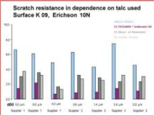
Figure 8: Different talc grades in a 18% talc filled copolymer, surface K 09.
