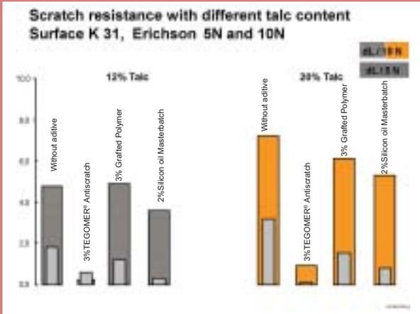
Figure 6: Scratch resistance depending on talc loading and additive technology.
